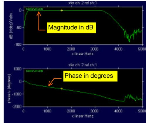
Figure 6 – Codec Frequency and Phase Response
