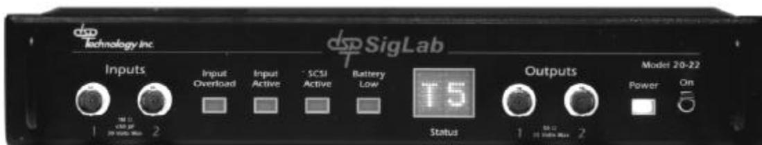
Figure 21 - SigLab Model 20-22 Signal Analysis System
