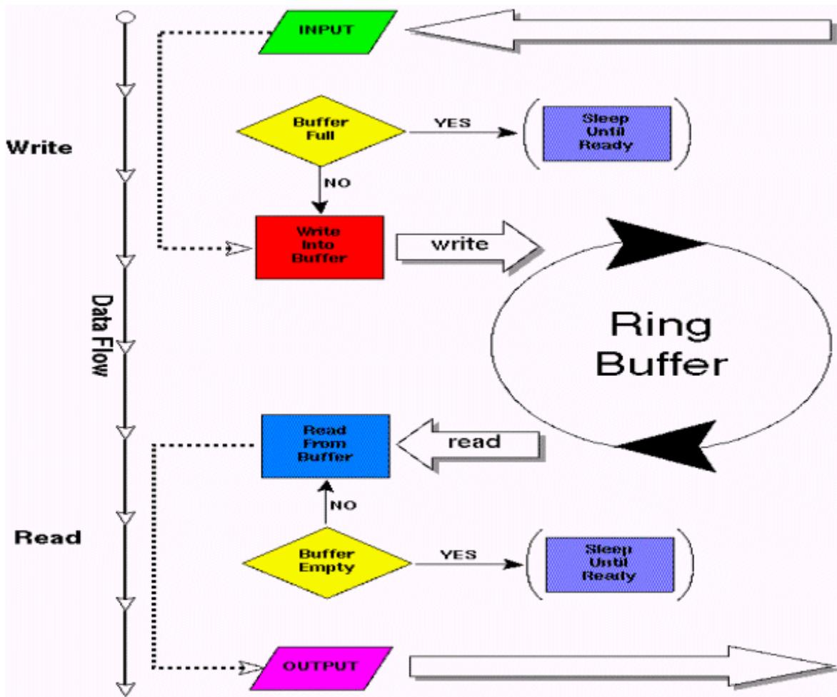
Figure 6. Acquisition Driver Ring Buffer
