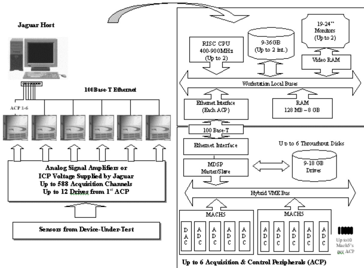
Figure 1. JAGUAR System Block Diagram
