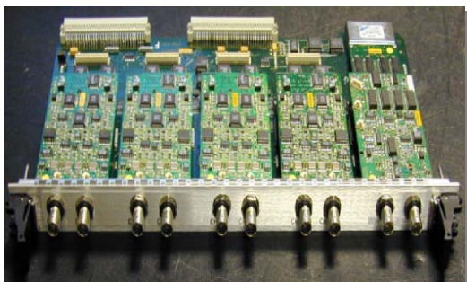
Example of measurement card with 8 Input and 2 Output capabilities
