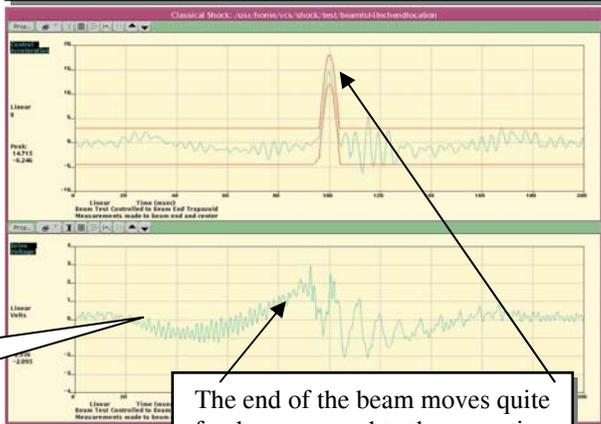
The end of the beam moves quite freely, compared to the mounting location. – The peak is correct and the test is a success!
