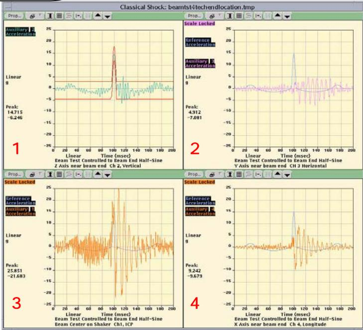
The graphic to the left **3** shows the pulse reference with the acceleration measured at the bolt location on the shaker head. Note the extraordinary demand placed upon the shaker to ensure that the beam end met the test criteria.
