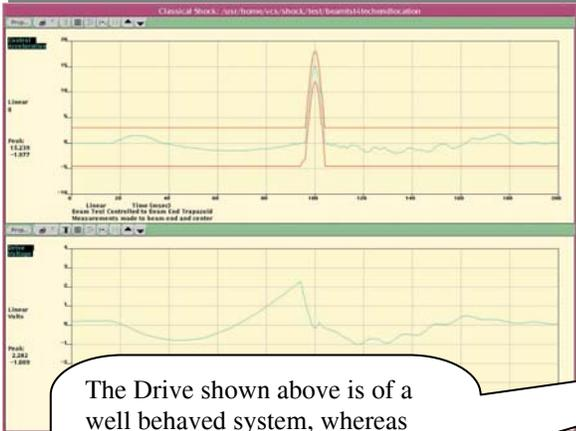
The Drive shown above is of a well behaved system, whereas the drive to the right shows a great deal of oscillation – required to make the shaker produce the correct pulse shape
