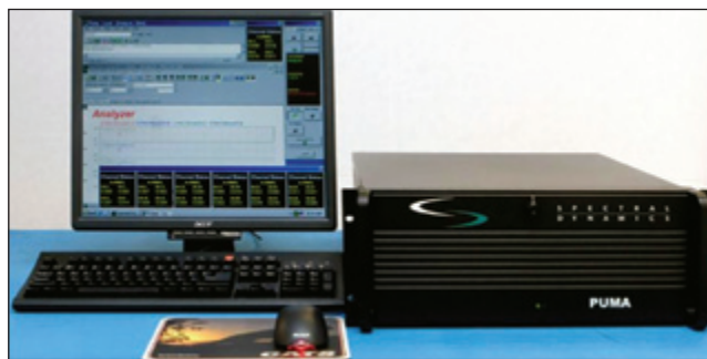
Figure 49. 32 Channel PUMA Control/Analysis System.
