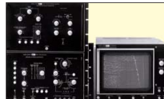
Elements of the AN/BQR-20: Spectral SD301 analyzer, SD13151 Spectrogram Display Control.
